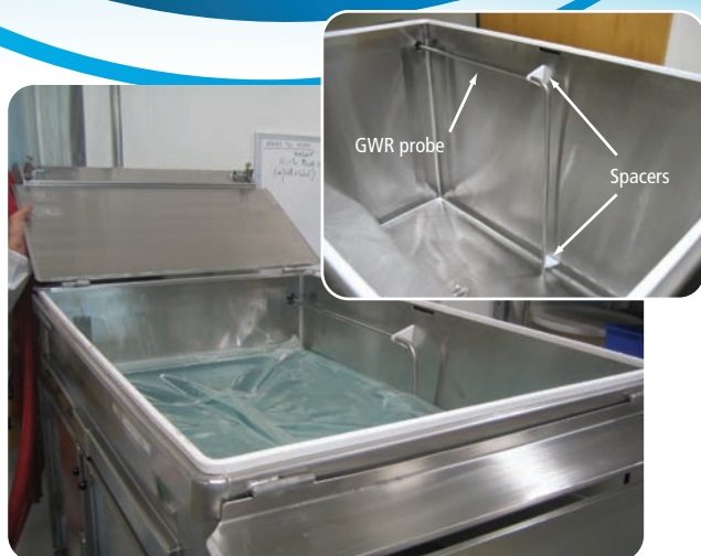
Figure 1. GWR probe installed in filled bioprocess container
